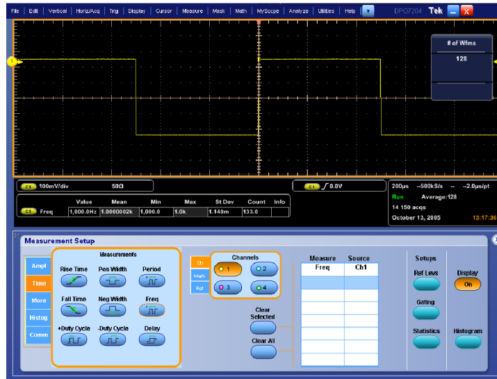
Figure 2-30: Measurement of probe compensator frequency
